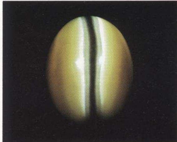
This glass imitation cat's-eye is made of fiber optic material.
