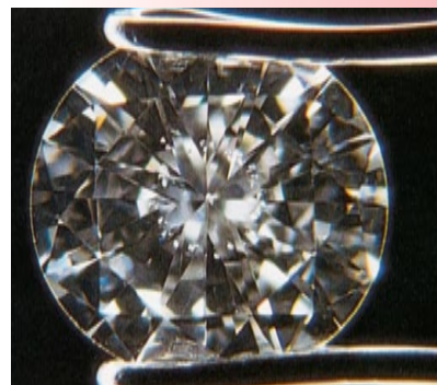
The position of just a few small inclusions (centered in the diamond) can have a significant effect on clarity. This is called a "reflector."
