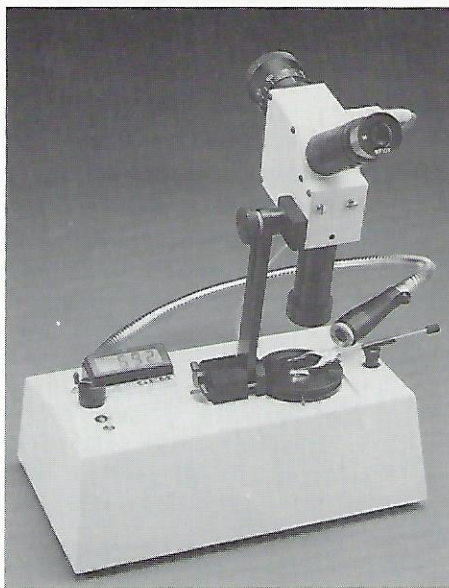
The DISCAN, a digital spectroscope, is the latest instrument produced by GIA GEM Instruments.
