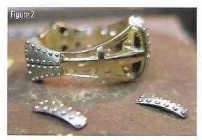
gold panels to be cast with the rivet holes in place, the walls of the holes were too thin to fill properly during casting. Linenberger edited his design, so that the small dimples in the surface where each rivet would go were now solid. When the panels were cast, he drilled each hole out with a #78 drill bit. The fit was so close that once the rivets were inserted, friction largely held them there during laser welding.
